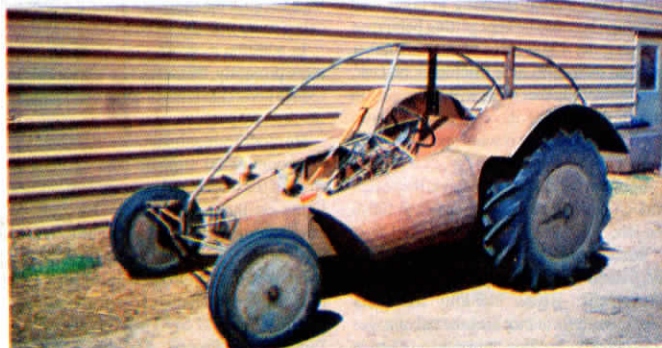
"Floating" tractor has narrow 15-in. front tires and large 24-in. lugged rear tires. A pair of hollow pontoons that bolt onto sides can be quickly removed.
