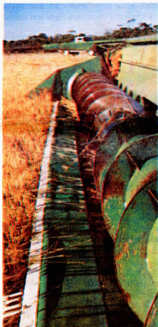
Vibra-Mat moves back, forth with sickle to transfer cut crop to auger without piling up on header platform.
