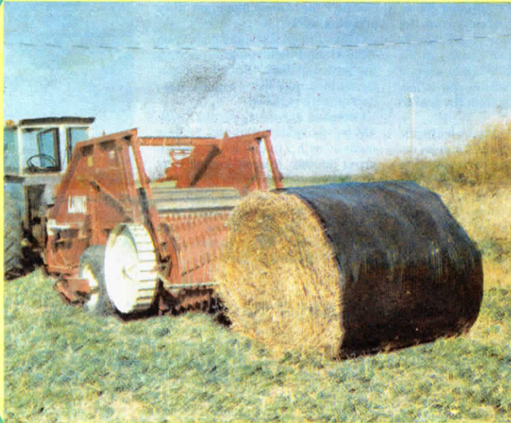
Front-mounted attachment on baler automatically wraps each bale in plastic in less time than it takes a conventional baler to twine-tie big bales.
