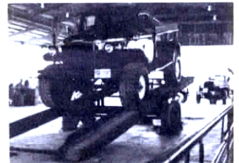
"Teeterboard" consists of pair of 27-ft. steel ramps mounted on tandem axle.
