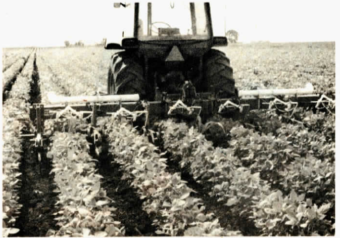
Central reservoir on each side pipes chemical to individual row units.
