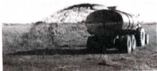
Milk tank spreader distributes manure over a 35-ft. area using a 4-bladed pto-powered impellor.
