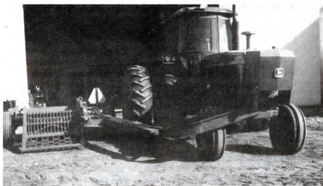
Side-mount lets Hagen pull picker alongside tractor and put a 3-pt. mounted rock digger on back.
