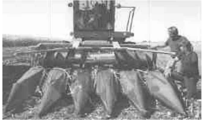
Kerkhoff built his own 22-in. head out of two used 4-row, 30-in. heads and mounted it on his self-propelled Deere 5460 power unit.
