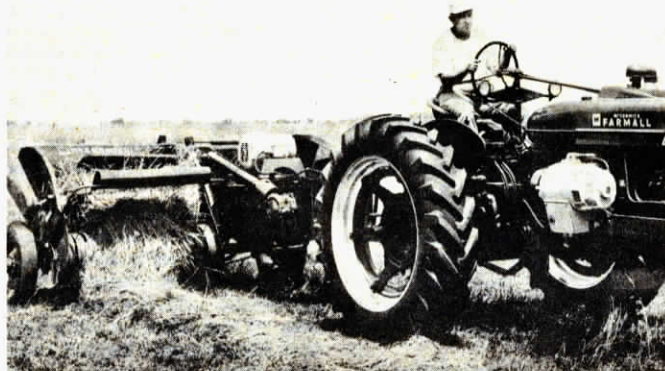
The IH Electral system, introduced in 1954, was designed mainly for use on Farmall Super M-TA and 400 tractors for use as a standby or portable electric power generator. However, it could also be used to power the model 55 baler. The baler was fitted with a 10 hp electric motor in lieu of a gas engine or pto drive.
