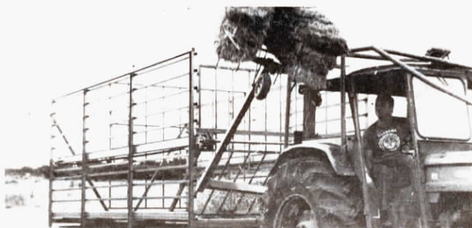
With flip of a switch, bale arm throws its load into trailing wagon and, in 3 seconds, is back on the ground.
