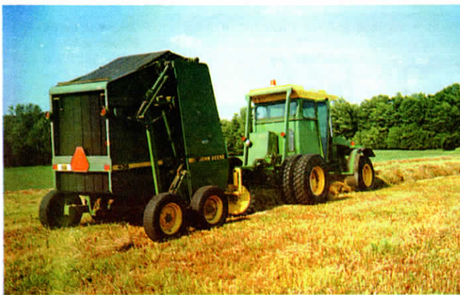
Speedy tractor was built on frame of a 1970 Chevrolet 3/4-ton pickup and has dual 20-in. lugged truck tires on rear axle with single 20-in. truck tires in front.
