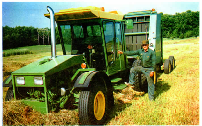
Krueger used the cab and hydrostatic transmission out of a Deere 7700 combine to build the tractor. Air bags off a semi truck mount under rear axle.
