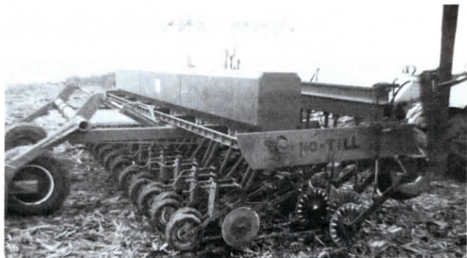
Disc openers and press wheels are supported by parallel linkage extending backward from toolbar under seed hopper. Hand crank on each row unit adjusts depth.
