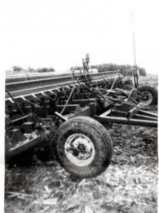
Hydraulic cylinders hooked to a nitrogen accumulator system from an old Oliver plow provide adjustable, cushioned down pressure on "bubble" coulters.
