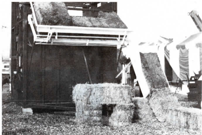
Stacked bales are loaded into rear of unit 72 bales at a time with fork lift equipped with squeeze. Destacker automatically aligns bales and unloads itself to feed bales into grinder, slicer, compactor or other processor.
