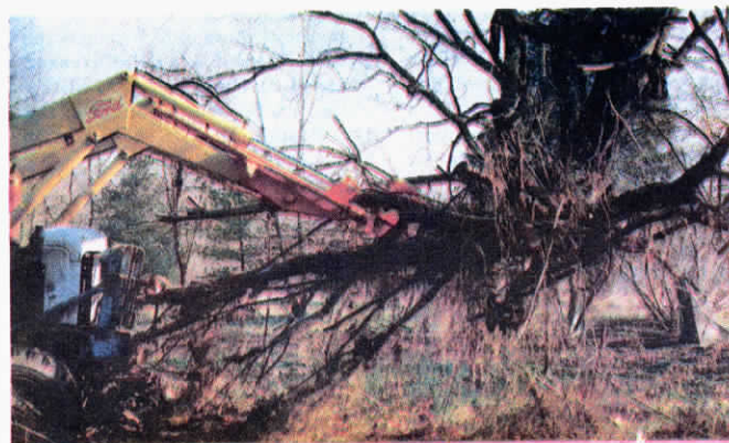
Splitter picks up logs for transport, or holds them at just the right height for cutting with a chainsaw.
