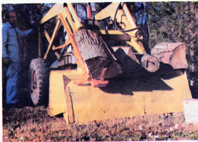
Loader-splitter weighs just 90 lbs. and installs quickly with two pins.
