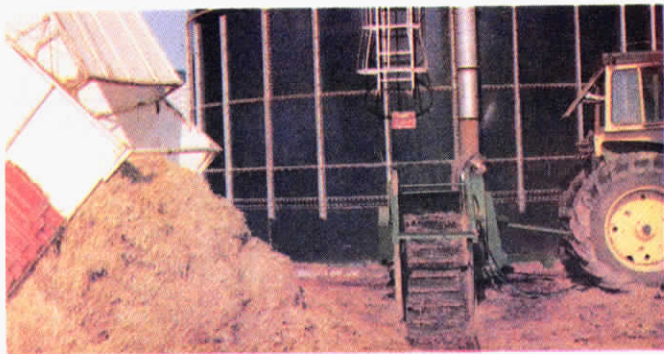
In grain or forage, this KIS conveyor will match the capacity of any silo blower, says Randy Bauer, inventor-manufacturer.
