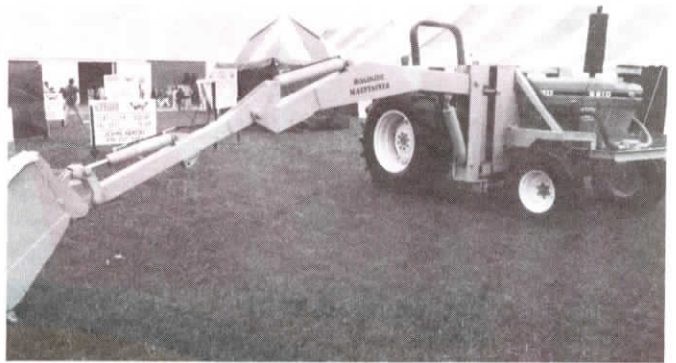
Side-mount backhoe swings 180° back and forth. Reaches out 18 ft. from tractor.
