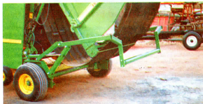
Bale kicker automatically activates when endgate opens.
