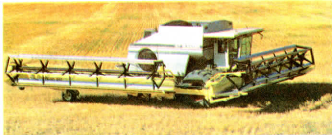
Outside header section folds back against combine for transport.
