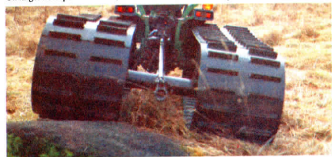
Key feature of Hansen's tracks is a T-bar which runs between the tracks, through the center of front and rear axles. No idler wheels needed.
