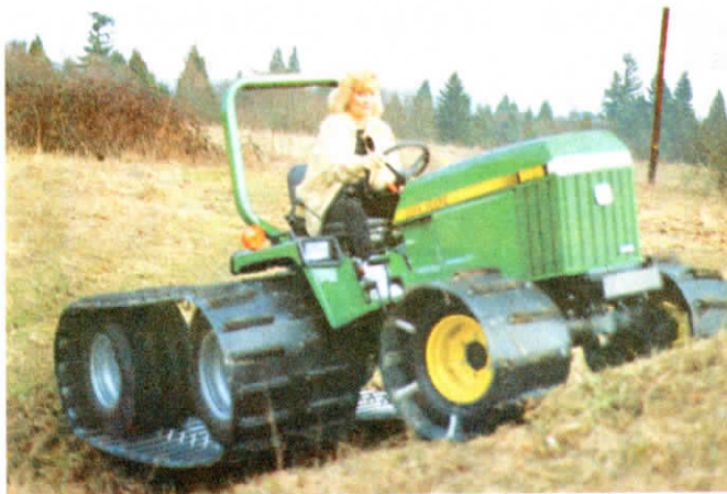
Add-on track system independently flexes in all directions when passing over rocks, ditches and other obstacles. High horsepower tractors can be fitted with a third axle.
