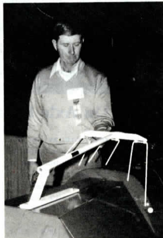
Swinging guard fingers raise up backwards to let stalks through.
