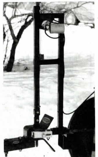
Electric motor, top, powers cable attached to hitch pin.
