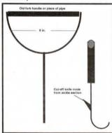
I made a handy hay hook that's comfortable and easy to use. I can hold it even with heavy mittens on. It's 6 in. wide and fitted with an old fork handle or a piece of pipe. Then I welded a sharp cut-off knife, made from a piece of an old sickle section, to the back of the hook to use to cut twine. Works good. (Donald Haman, Rt. 3, Box 71, Wadena, Minn. 56482 ph 218 385-3677)
