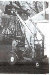
I built this little loader tractor 20 years ago and it's still working. It has a 4-ft. bucket, a Ford pickup rear end, a '41 chevy transmission, a 4-cyl. Continental combine engine, live hydraulic pto on front to run augers and elevators, and front wheels off a Buick. It's been used primarily for cleaning calf and hog barns. We call it the "Budcat". (Orrin "Bud" Davis, Rt. 2, Box 108, Lake Park, Minn. 56554 ph 218 532-7858)
