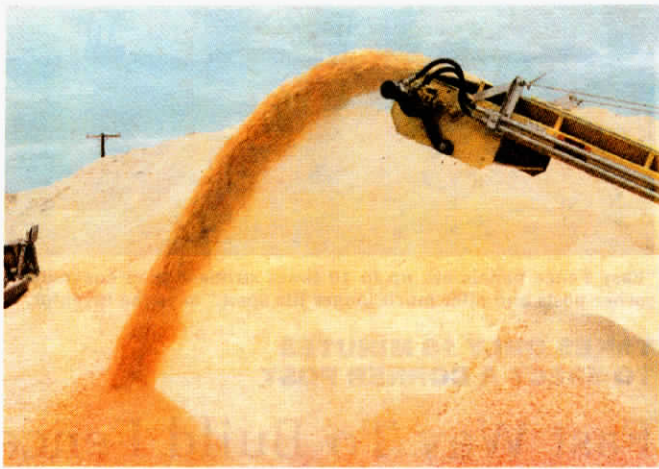
The 54 in. model cracks corn kernels open, without creating fines, at the rate of 150 tons per hour.
