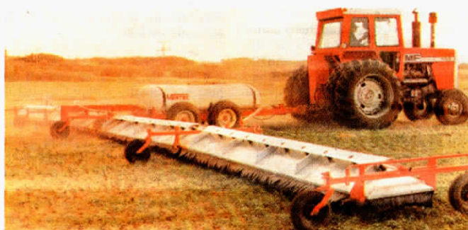
Airfoil on top of galvanized shroud directs air flow down along the back to eliminate turbulence and thus avoid problems with drift.
