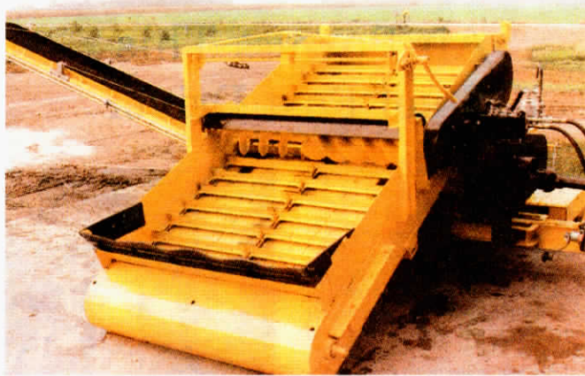
Conveyor carries grain up and dumps it into the "particulator's" spiked cylinder.
