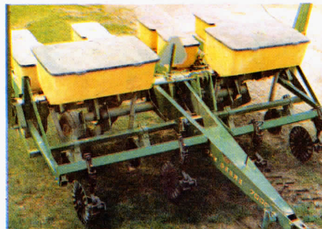
Second add-on planter is mounted between the lift wheel and hinge point.
