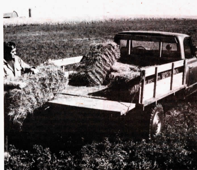
Standard bed is 8 ft. long with 20 in. high sides and a drop tailgate. Other sizes can be ordered custom made.
