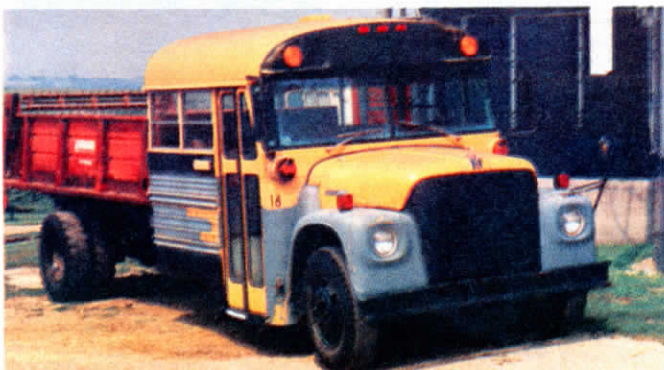
Bus-spreader's 5-speed transmission is geared low enough that Olson can drive at tractor speed in the field.
