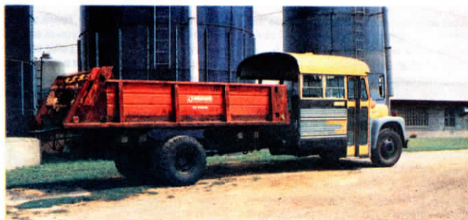
Olson used a chop saw blade mounted on a skill saw to strip away the body of the bus before mounting the spreader box on the chassis.
