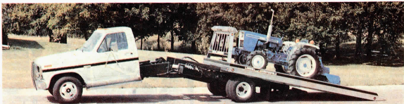
"It's great for hauling low-slung equipment," says Larry Holmes of Landoll's Centerfold "drive-on" flatbed which tilts for loading, unloading.
