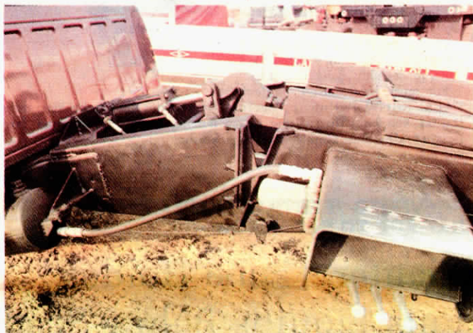
Hinge is installed by splitting truck just behind cab.
