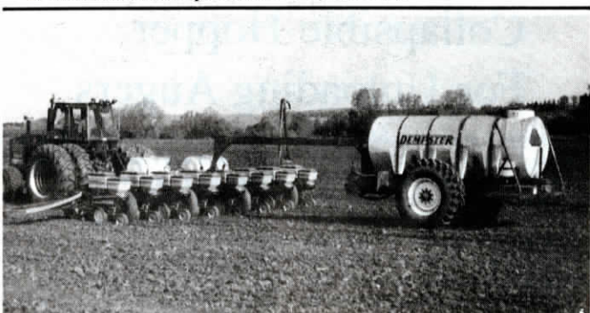
Dempster Tracker's narrow wheels fit between rows. Sprayer is powered by a ground-driven pump.
