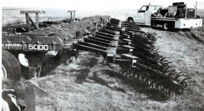
You can pull "Active Harrow" behind any tillage tool or use it by itself.
