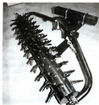
Because the end of each spike is straight up as it leaves the soil, straw and weeds don't wrap around drum.
