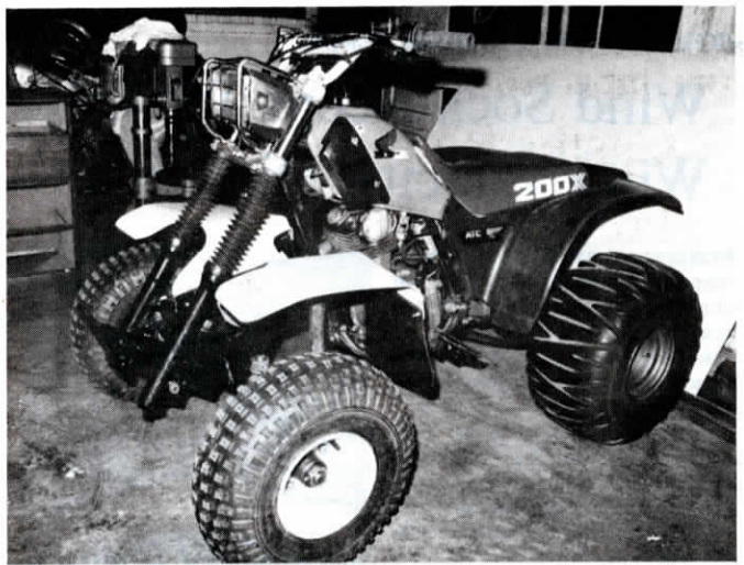
To install, you remove the 3-wheeler's front tire and fender and then fasten a bracket with a U-clamp onto the frame just above the motor mount.
