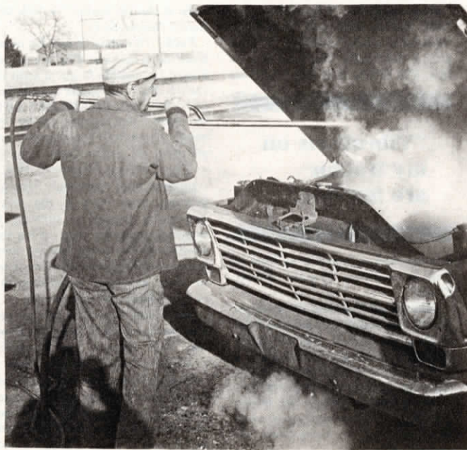
Kleen Gun harnesses exhaust air generated by your pickup or tractor engine. It can be hooked up to siphon cleaning liquid from a container. Or, you can use it as a "dry" cleaner to blow out radiators, filters, etc. Can also be used to warm cold motors, remove ice from windshields, or to spray livestock.
