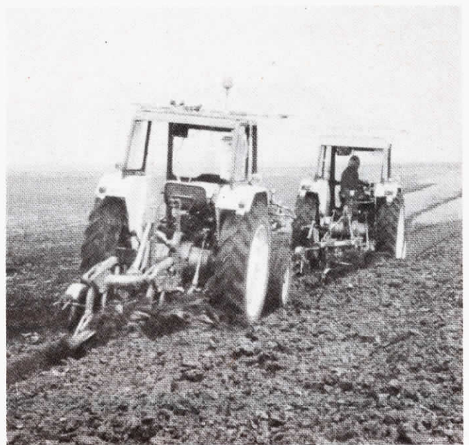
One driver (on front or master tractor) controls both tractors. Engine speed of slave tractor and its distance from master tractor is maintained automatically.
