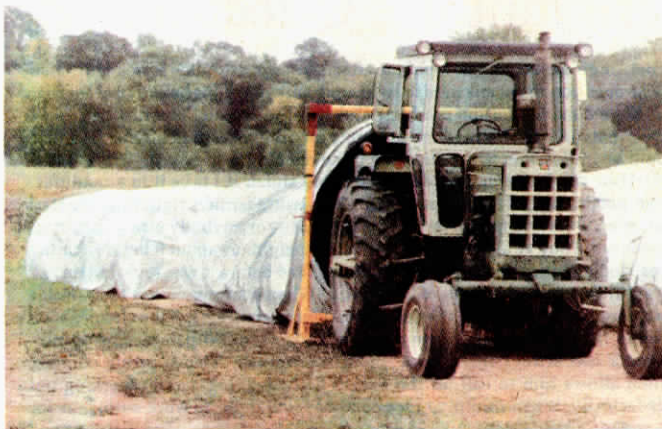
Tractor backs into "bagger" to load big bales into the 200-ft. long bag.
