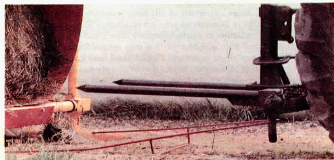
As 3 pt. is lowered to set the bale inside the ring, it hooks into V-shaped tongue of bagger. Tractor then pulls bagger forward about 5 ft. to position it for next bale.
