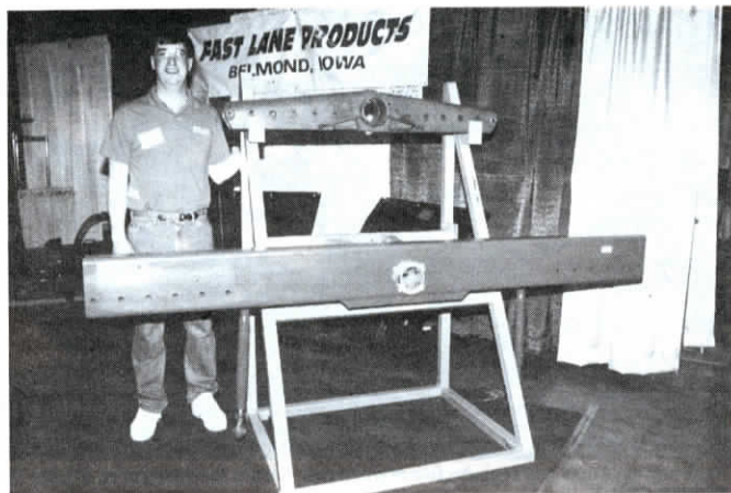
New axle (bottom) is wider and heavier than original (top).
