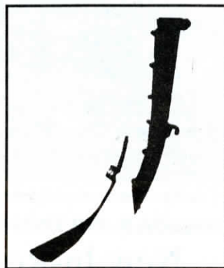
Curved nylon paddle fastens to back of seed tube with two tie straps.
