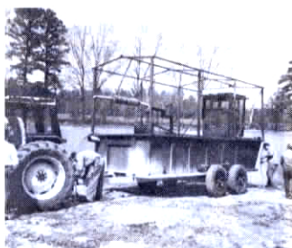
Bradsher built "sand harvester" out of an old garbage dumpster and a Gleaner combine cab.
