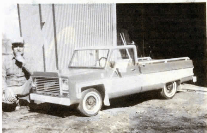
Neuhalfen's "mini" pickup is powered by Briggs & Stratton 8 hp gas engine and has an automatic transmission and power steering.
