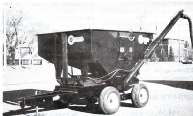
Heavy-duty walking beam tandem axle chassis is made out of 6-in. sq. tubing.
