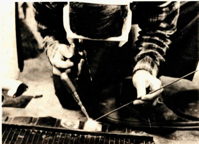
Except for aluminum, flux is not normally required with the Dillon torch.
