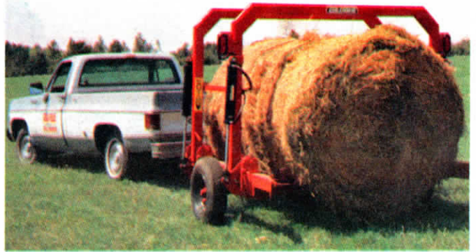
Open frame trailer has arched overhead frame. Four hydraulic cylinders, two on each side, lower the side rails down to ground to pick up bales.
