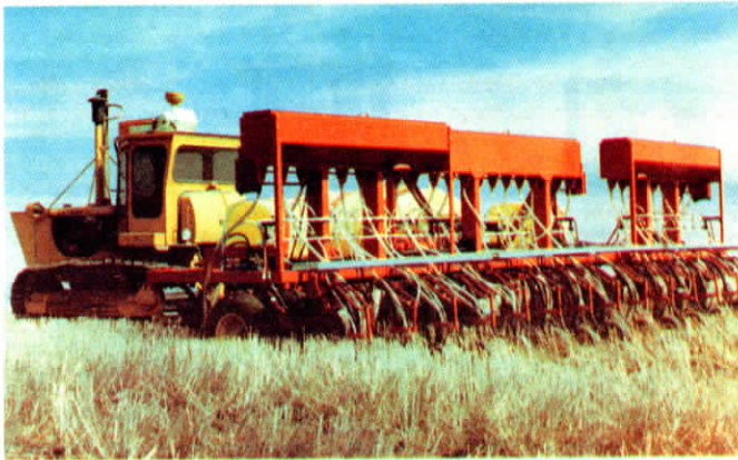
The 29-ft. drill has 11-ft. center section and two 9-ft. wings that fold up for transport.
