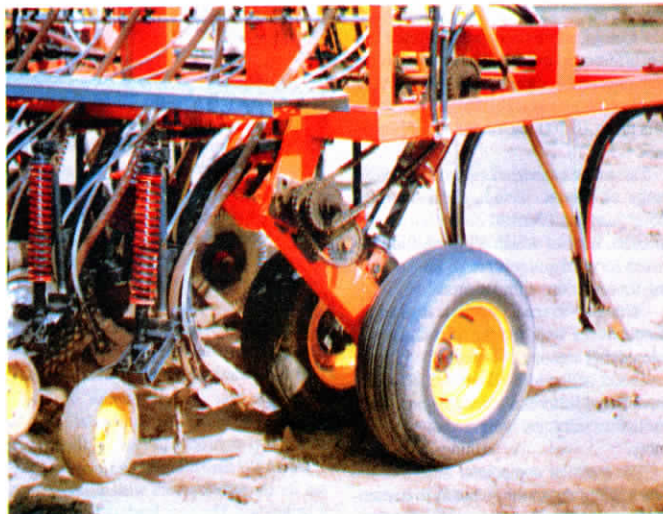
Special-built chisel plow points have seed distributor plates on back that deposit seed on ledges in furrow. Fertilizer is deposited in bottom of furrow.
