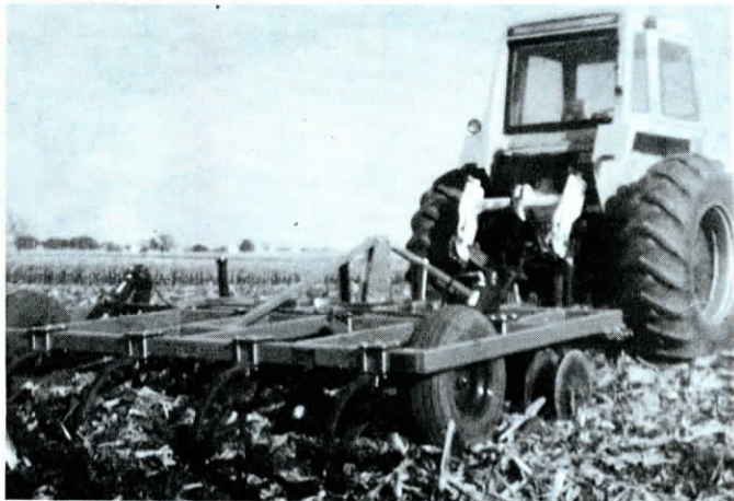
New Soil-Master is equipped with 20 in. disk "slicer" blades.
