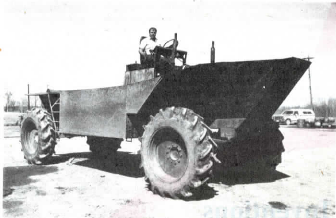
The 4-WD, 4-wheel steer tractor has 24 gears thanks to its doubled-up transmission.
