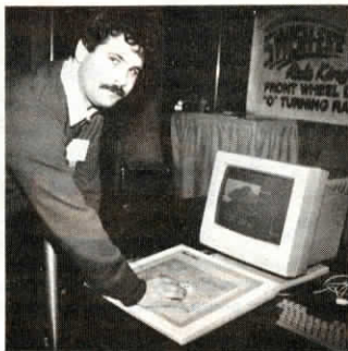
Field boundaries, soil type lines and other information are traced on the graphics tablet and appear simultaneously on the computer screen.
