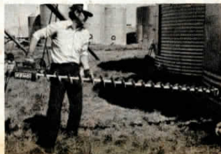
You move the 6 in. dia. flighting and power head from bin to bin.
