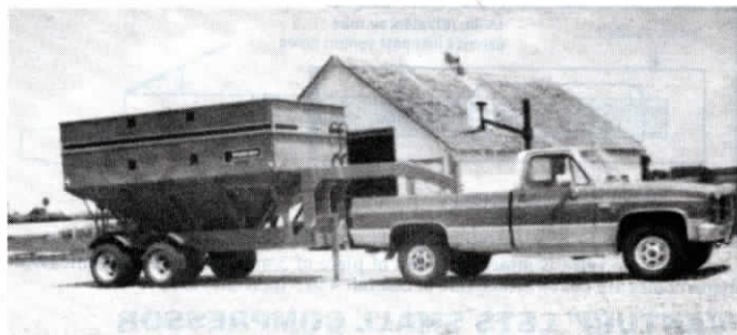
Wagon gear consists of 8-ft. gooseneck and 14-ft. tandem axle frame that bolts onto each corner of standard center dump grain box.
