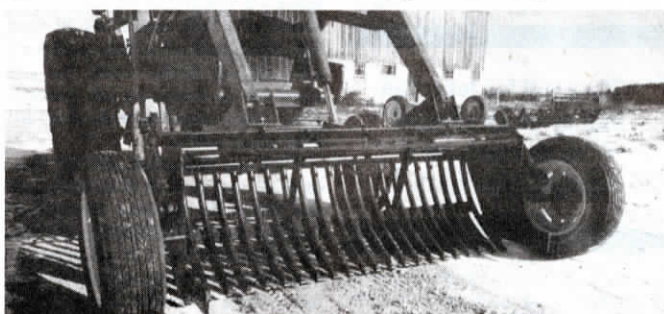
Rock picker has steel teeth spaced 2 in. apart that skim ground to scoop up rocks.
