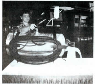
30-gal. tank has 10 times as much capacity as a conventional fire extinguisher.
