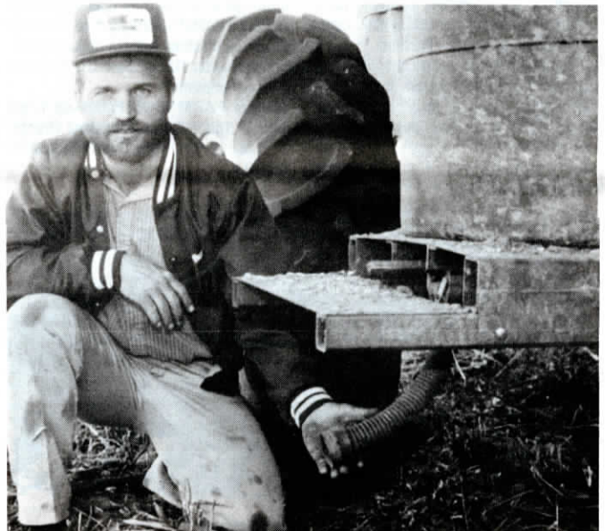
Andre positions 55-gal. barrel directly behind front drive wheels. Seed drops through rubber tube into wheel tracks and is worked into soil by lugs on rear tires.
