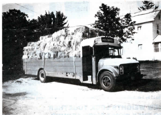
The seats and top 3 ft. of the bus were cut off back from just behind the driver's seat.
