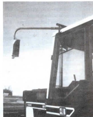
The 6 by 12-in. mirror mounts on sliding support tube.
