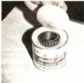
Two cone-shaped parts "sandwich" bearing to evenly pack grease into rollers.
