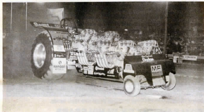
The 9,000 hp tractor pulls a 50,000 to 80,000-lb. sled along a 300-ft. track, using up to 20 gal. of fuel in less than 20 seconds.
