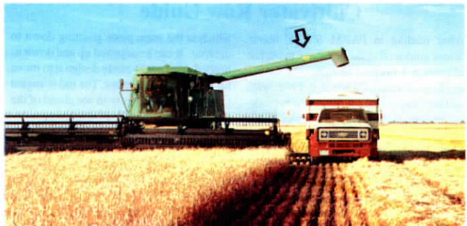
Extender gets auger out beyond end of combine header so trucks don’t have to worry about running into back of header.
