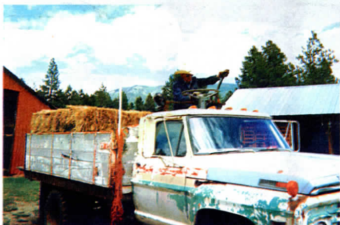
Pemle drives truck while standing on flatbed behind cab, using steering wheel mounted on cab roof and remote clutch and throttle controls.
