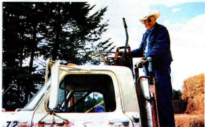
A flexible cable runs from foot clutch up to remote clutch lever mounted on top of cab. A choke cable also runs from top of cab to throttle lever on carburetor.
