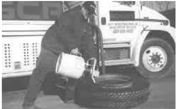
Air tank blasts air into tire to instantly snap beads into place. To use, you slip unit's wide, flat spout between bead and rim and push a button to release the air.
