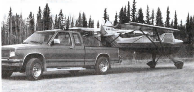
When wings are folded, plane can be towed behind your car or pickup.
