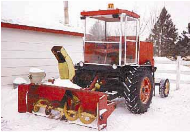
Fleckenstein's rig consists of an 8-ft. snowblower mounted on a Gleaner A combine.
