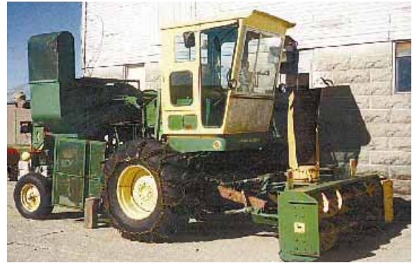
Baldwin mounted an 8-ft. two stage Deere snowblower on a Deere 95 combine.
