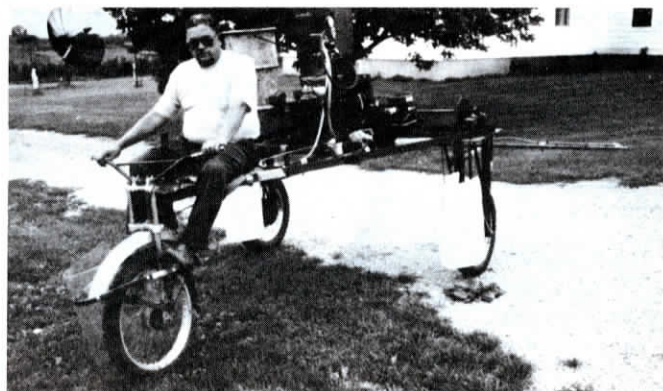
Electric broadcast seeder mounts on back of home-built 3-wheeler.
