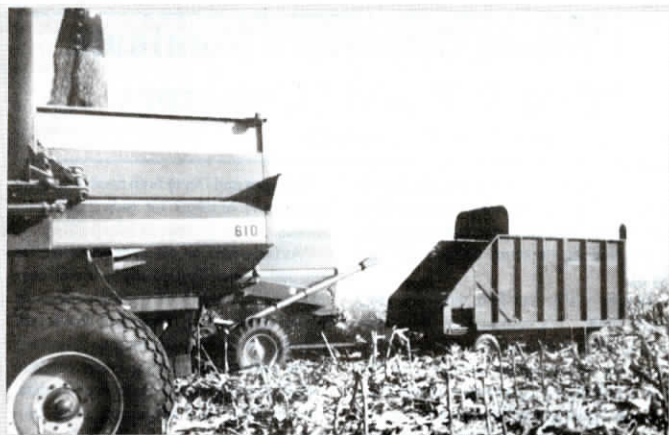
A silo blower mounted on back of Hibbs's Deere combine blows cobs into a tow-behind wagon. He sells cobs to a nearby processor.
